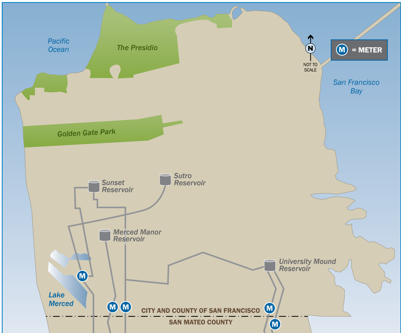
Figure 7: Distribution System Area and Metering Locations
