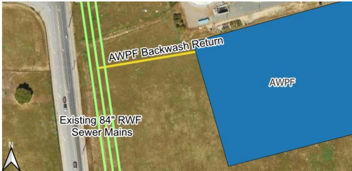
Figure ES.7 AWPF Waste/Backwash Return Pipeline Alignment
