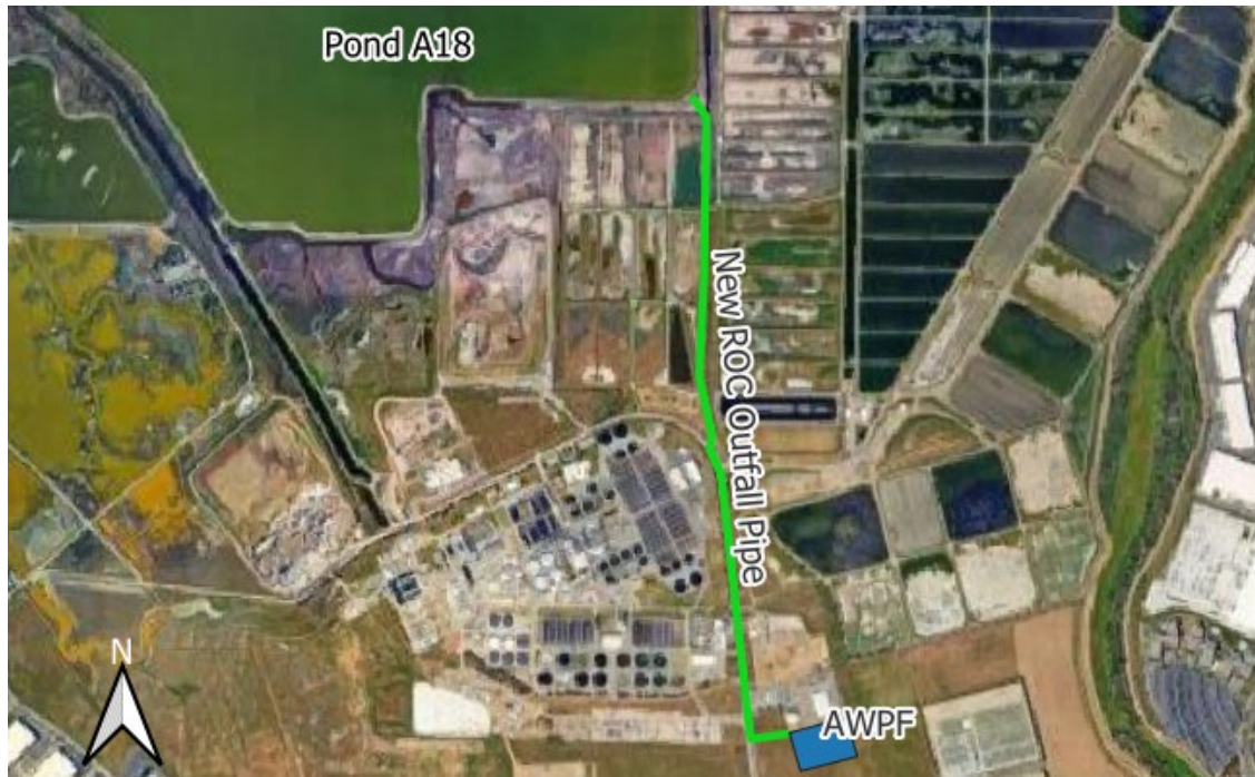
Figure 4.11 ROC Pipeline Alignment to New Outfall
