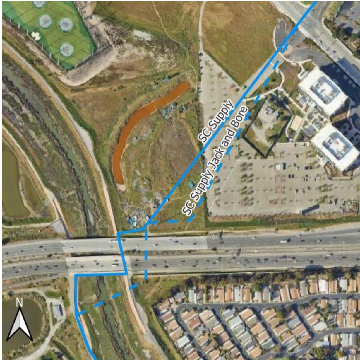
Figure 4.6 Two Alignment Options for the Santa Clara Finished Water Pipeline Crossing at Highway 237 and the Guadalupe River
