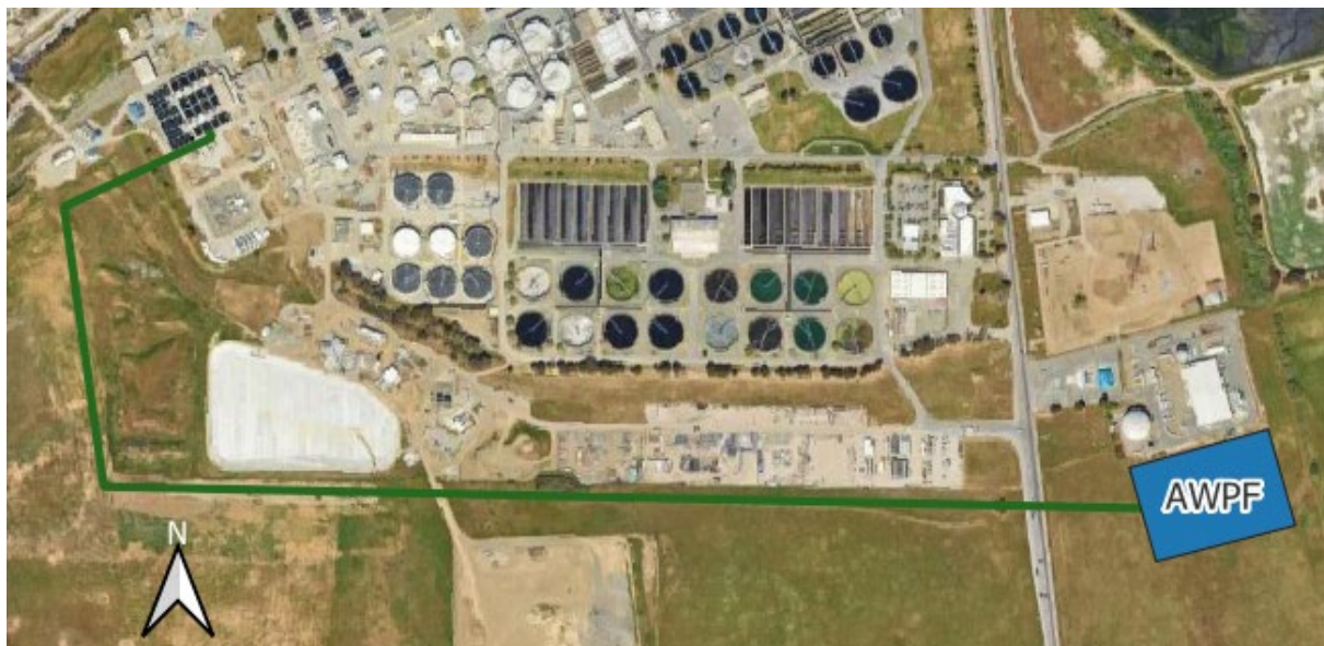
Figure ES.4 AWPFF Feedwater Pipe Alignment
