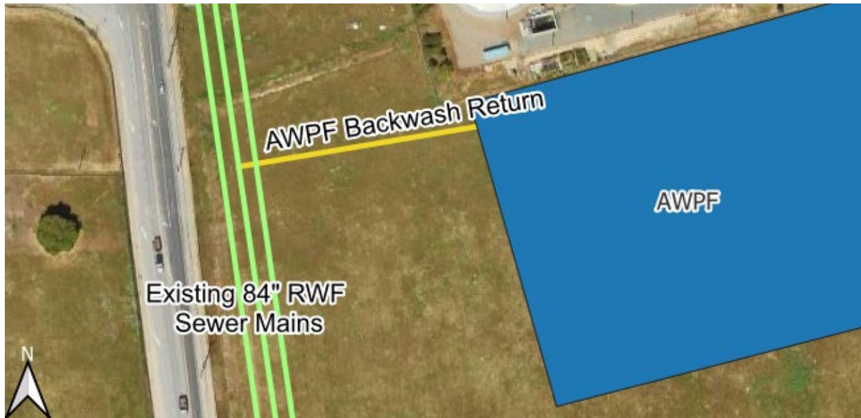
Figure 4.12 AWPf Waste/Backwash Return Pipeline Alignment
