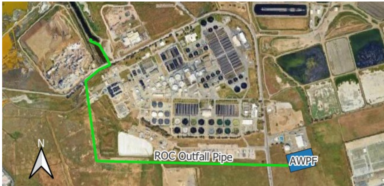
Figure 4.10 ROC Pipeline Alignment to Existing RWF Outfall
