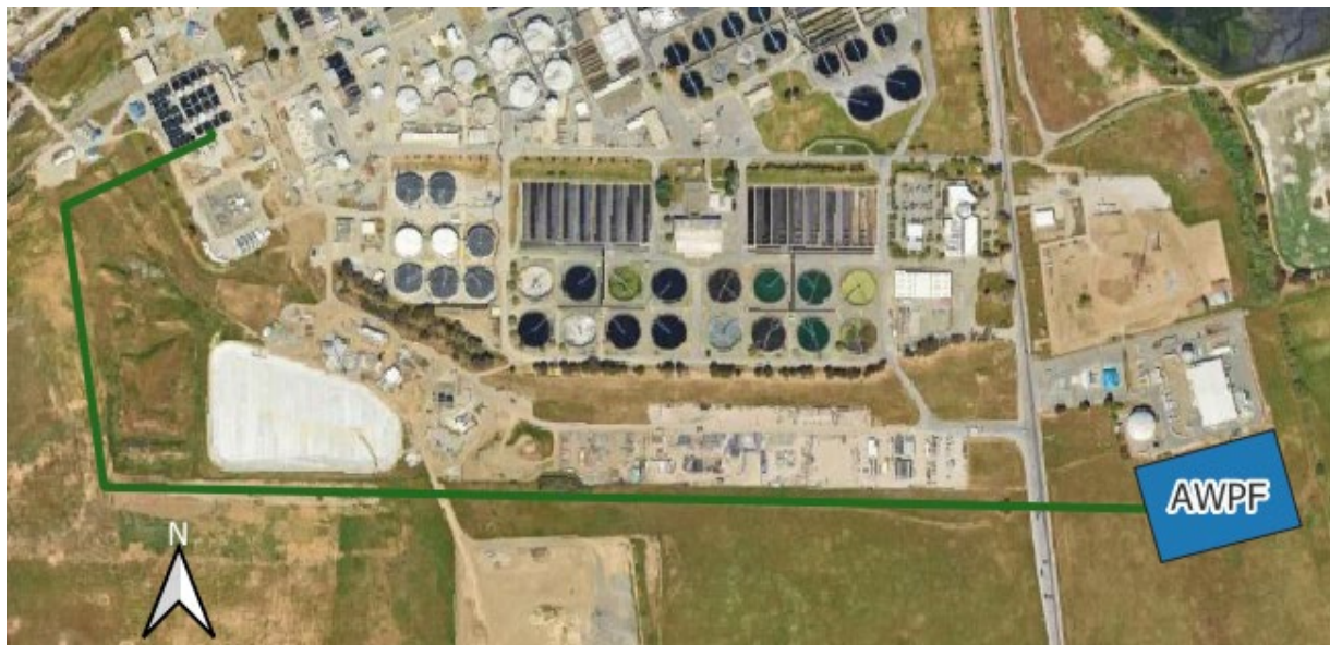
Figure 4.1 AWPF Feedwater Pipe Alignment
