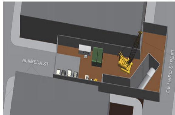
3D graphic of proposed rotation shaft site for the tunnel boring machine at Alameda and De Haro
