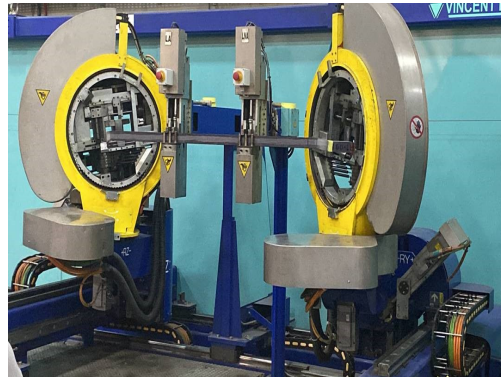
Generator Winding Bars being formed in factory
