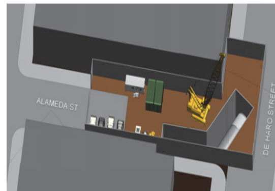
3D graphic of proposed rotation shaft site for the tunnel boring machine at Alameda and De Haro
