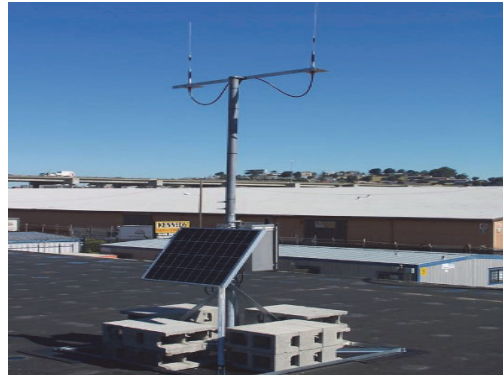
AWMP Data Collection Unit on the roof of the CDD Operations Building
