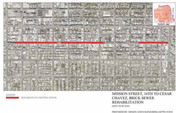
Schematic for Large Sewers – Mission BSR
