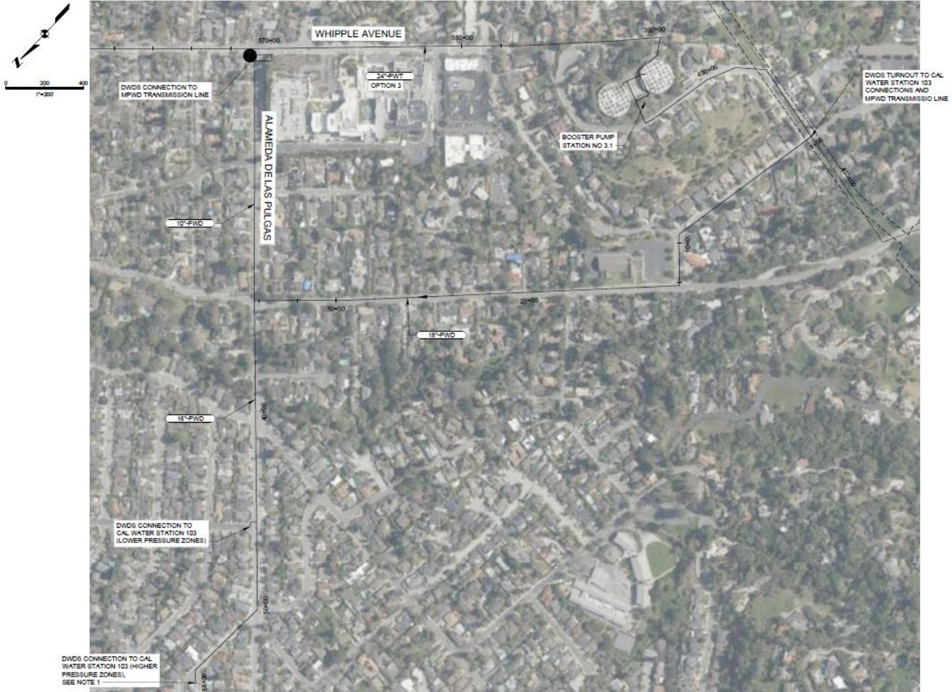
Figure 3-14: RWC Sequoia Tanks, Cal Water Station 103, and MPWD Transmission Line Approximate Tie-in Locations and Distribution Pipeline Extensions for Purified Water Transmission Alignment Option 2
