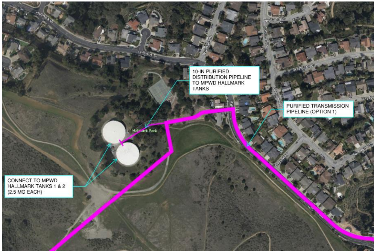
Figure 3-7: MPWD Hallmark Tanks Approximate Tie-in Location and Distribution Pipeline Extension for Purified Water Transmission Alignment Option 1
