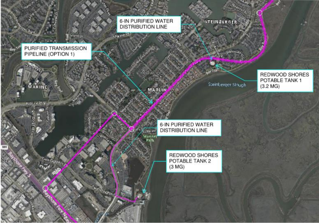
Figure 3-5: Redwood Shores Potable Tanks Approximate Tie-in Location and Distribution Pipeline Extensions for Purified Water Transmission Alignment Option 1
