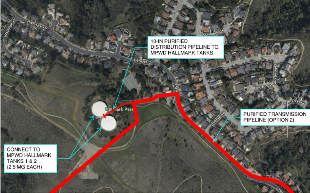
Figure 3-11: MPWD Hallmark Tanks Approximate Tie-in Location and Distribution Pipeline Extension for Purified Water Transmission Alignment Option 2
