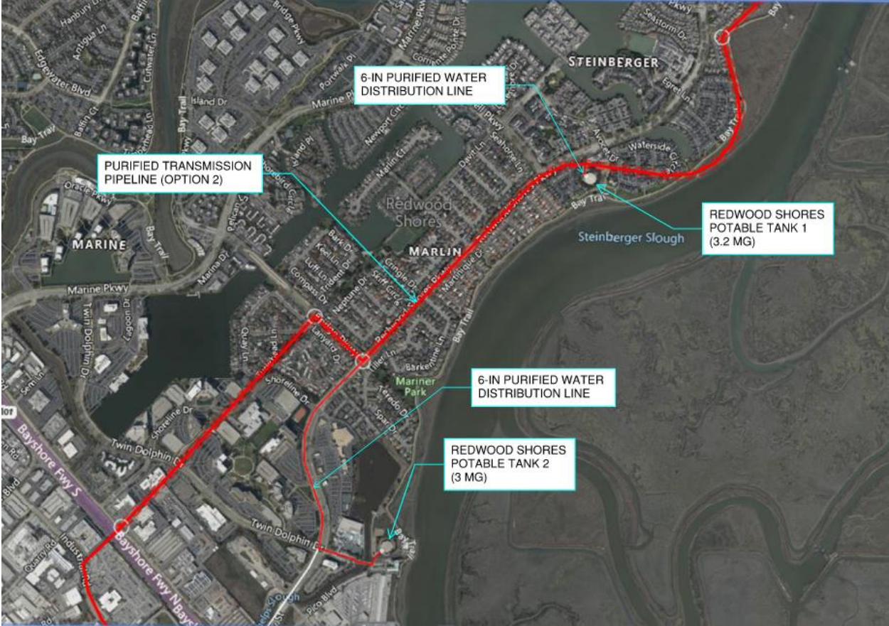
Figure 3-9: Redwood Shores Potable Tanks Approximate Tie-in Locations and Distribution Pipeline Extension for Purified Water Transmission Alignment Option 2
