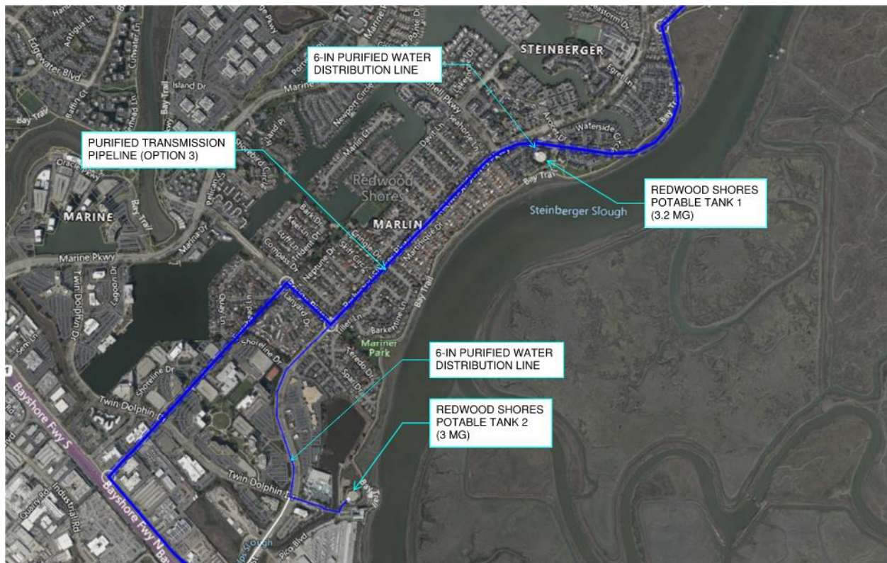
Figure 3-13: Redwood Shores Potable Tanks Approximate Tie-in Locations and Distribution Pipeline Extension for Purified Water Transmission Alignment Option 3
