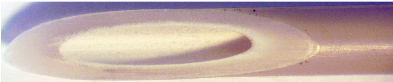
Stereoscope image (20x) of the filtrate side of a fiber from Sample 1
