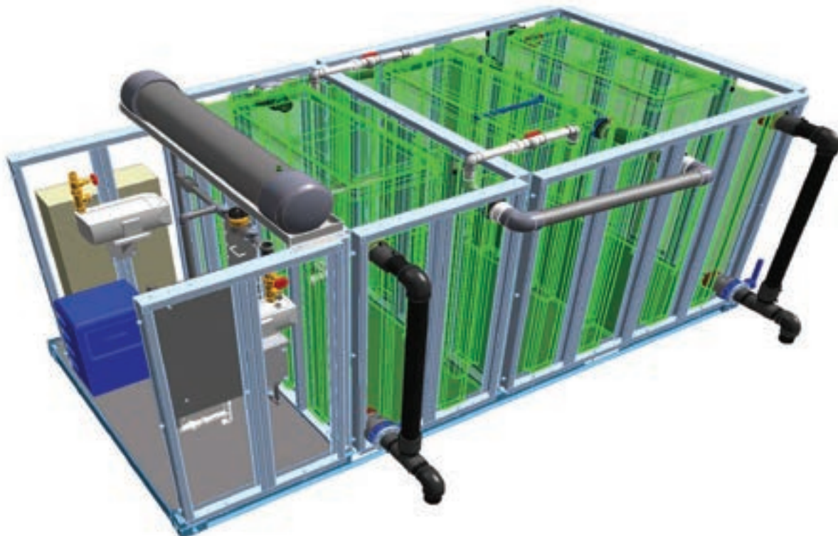
A rendering of the treatment system at 181 Fremont Mixed-use Tower (image courtesy of PHOENIX/Aquacell)
