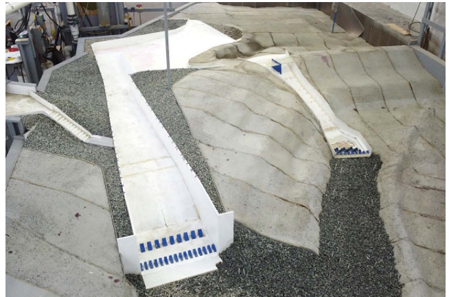
Physical Model of the Moccasin Dam Spillway Conceptual Design
