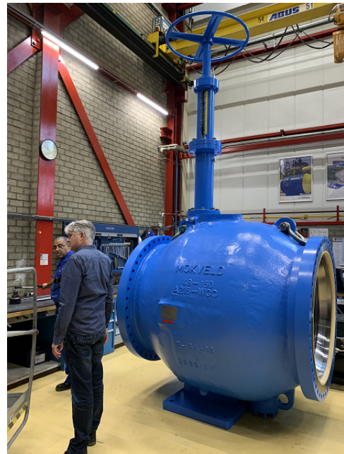
Axial Control Valve Similar to What is Planned for Use in the Moccasin Powerhouse Bypass Upgrade Project
