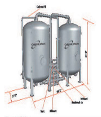
Typical Granular Activated Carbon Vessel that may be Used to Treat Regional Groundwater
