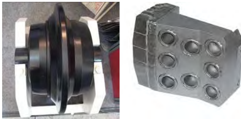
Figure G-4: Disc Cutter (L) and Scraper (R)
