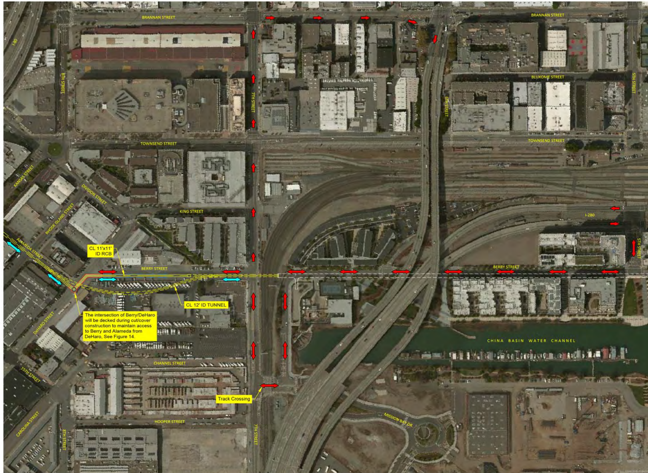
Figure 17 Construction Traffic Route – Cut-and-Cover to I-280
