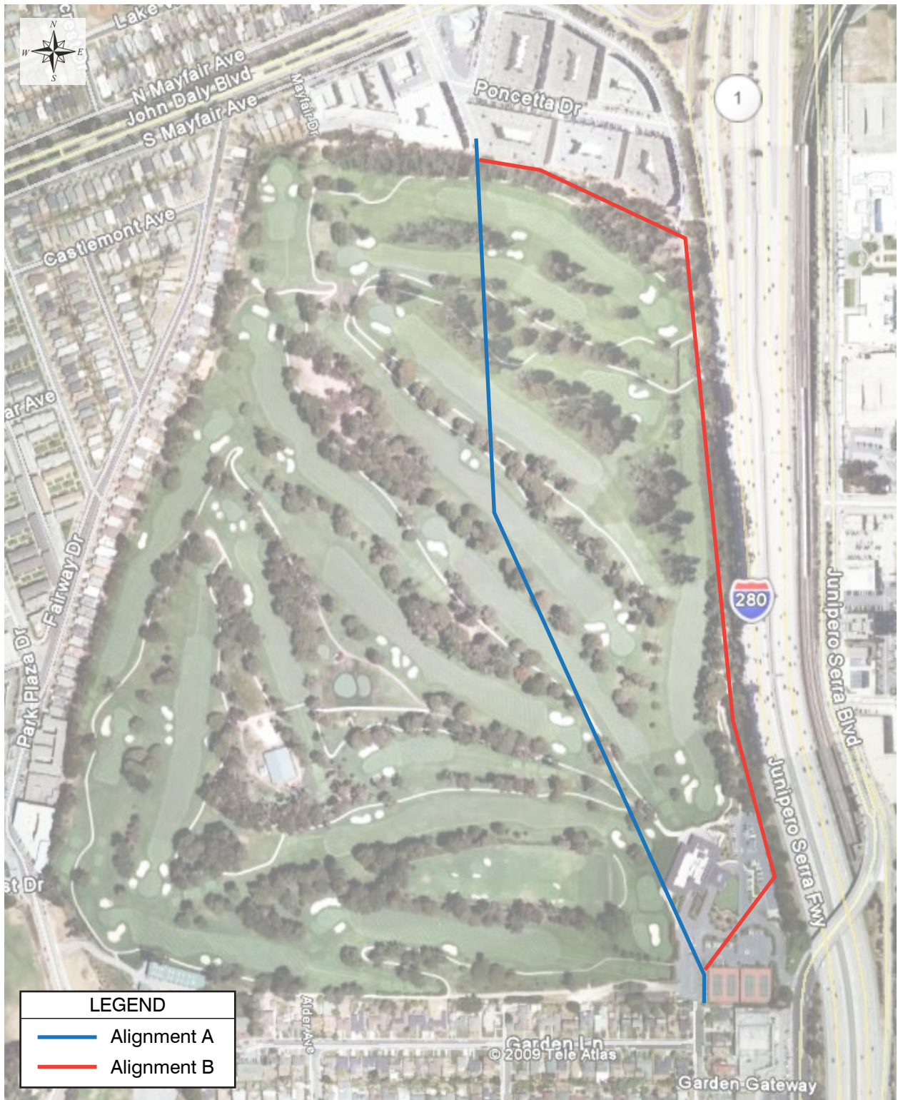
Figure 1.5 SEGMENT NO. 2 CITY OF DALY CITY RECYCLED WATER TRANSMISSION MAIN CORRIDOR STUDY
