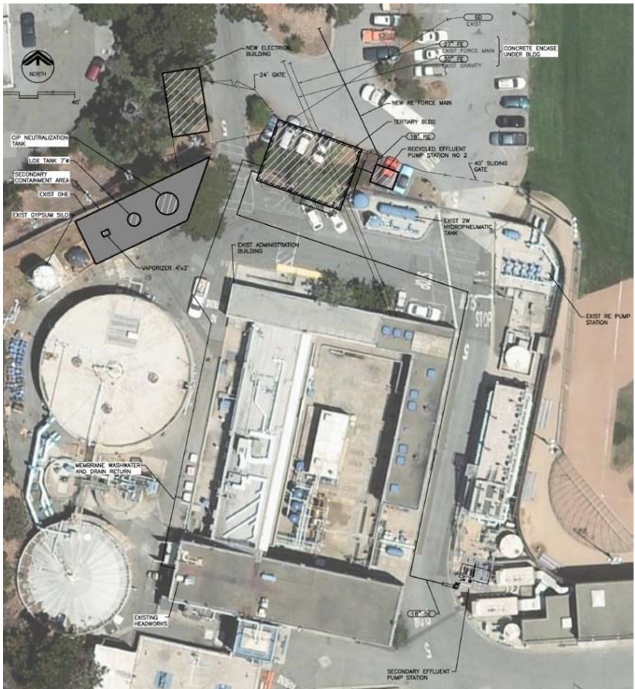
Figure ES.5 PROPOSED LAYOUT FOR TERTIARY EXPANSION CITY OF DALY CITY COMBINED RESULTS OF THE RECYCLED WATER TREATMENT AND DELIVERY SYSTEM EXPANSION FEASIBILITY STUDIES
