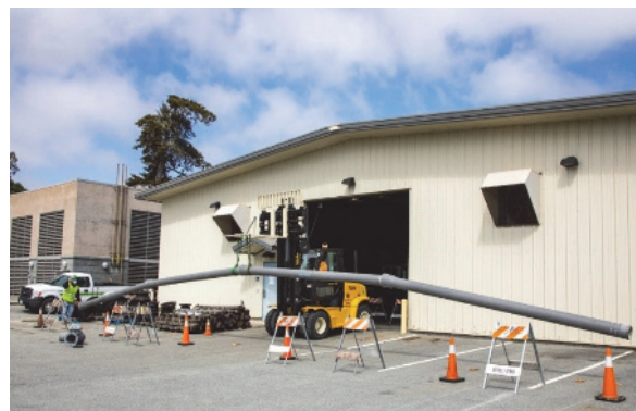
Earthquake Resistant Ductile Iron Pipe with flexible joints that may be used in the PEFWS projects
