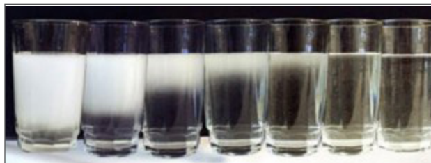
Temporary presence of air in water due to changes in water temperature and pressure (Source: Massachusetts Water Resources Authority, 2020)
