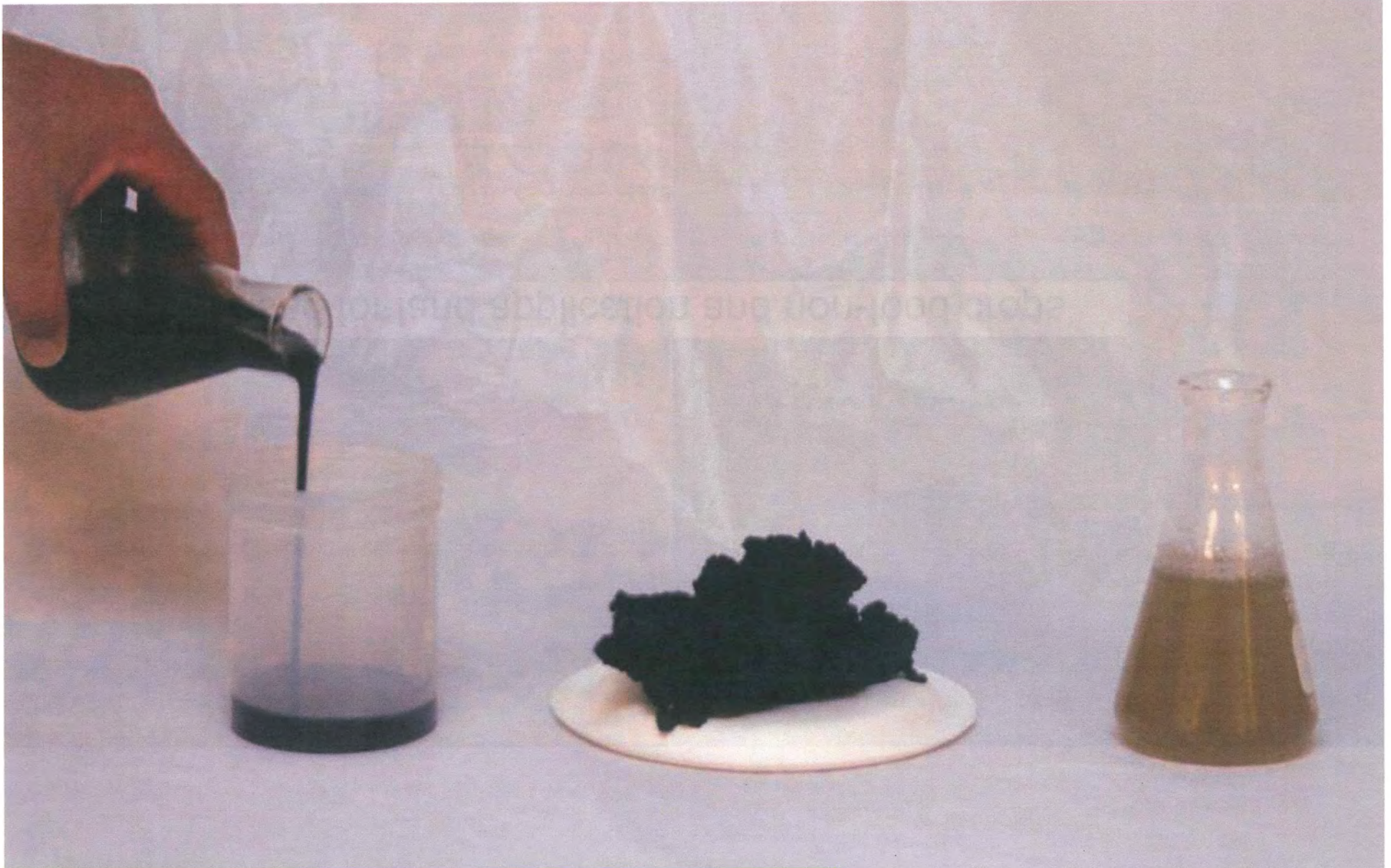
Biosolids (Byproduct of Digestion)
