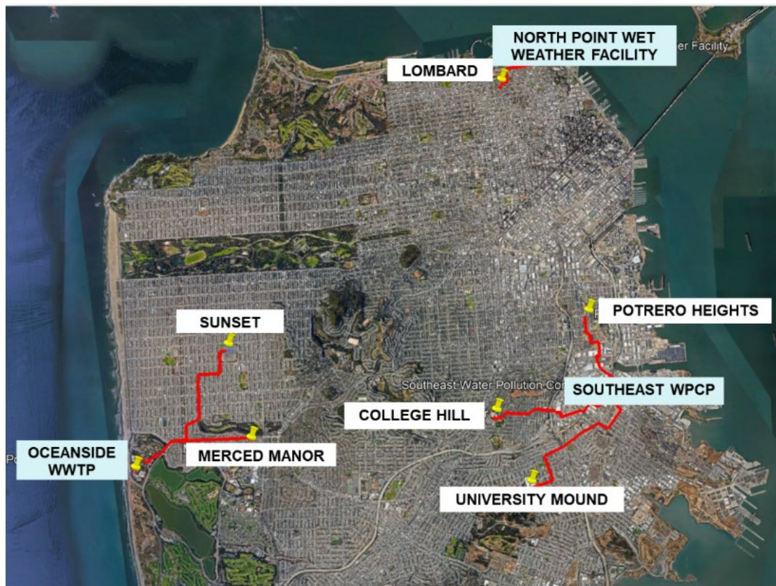
Figure 2.4 Potential Pipeline Paths between WWTP and Drinking Water Reservoirs (AWPF locations not considered here)
