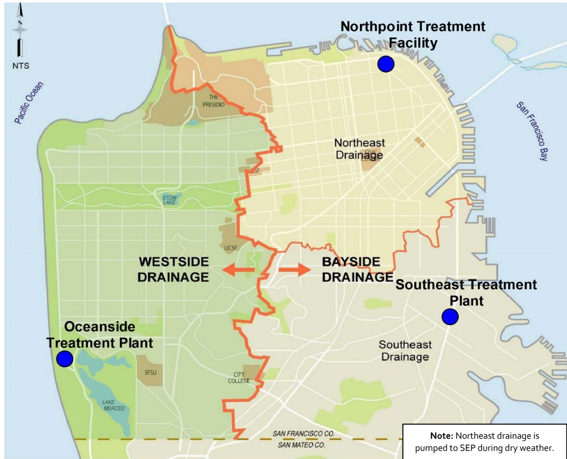
Figure 2.2 San Francisco Wastewater/Stormwater Drainages Areas (Source: Adapted from SEP NPDES Permit No. R2-2013-0029)
