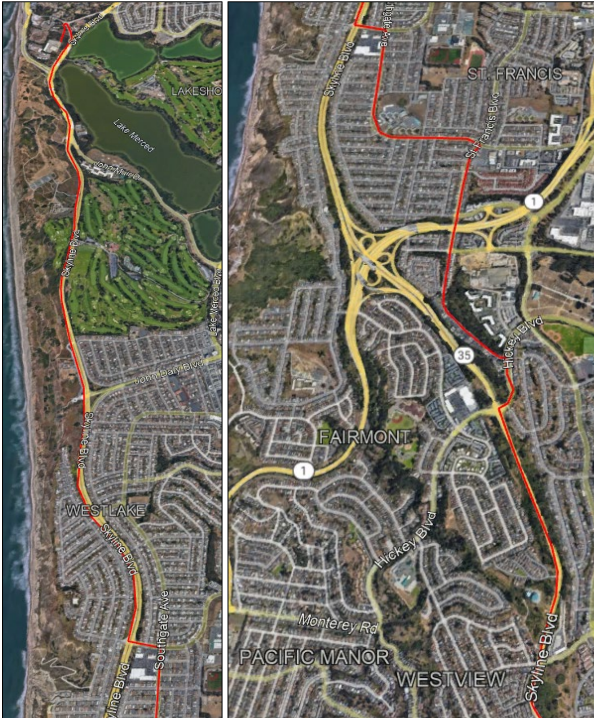
Figure 2 Pipe Alignment Details 1 and 2 of 3 to Convey Flows from OSP to San Andreas
