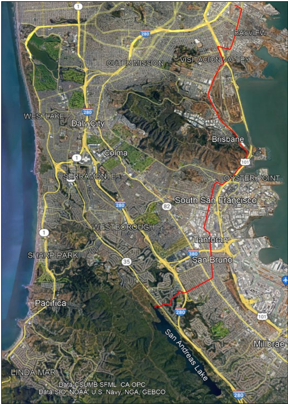
Figure 5 Pipe Alignment Overview to Convey Flows from SEP to San Andreas Reservoir
