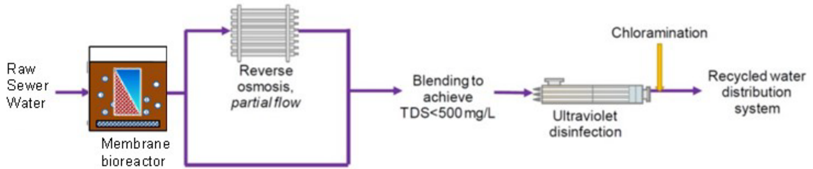
Figure 4-1. Conceptual Treatment Train for a Satellite Treatment Facility Generating Recycled Water from Raw Sewage
