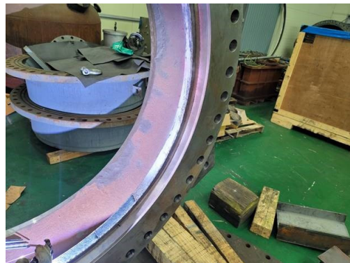
Components of 66-inch Butterfly Valve being assembled in factory
