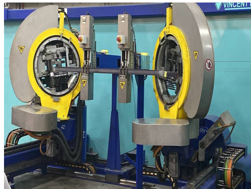
Generator Winding Bars being formed in factory
