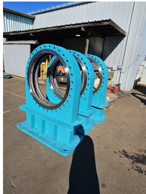
HH-1005 Factory Fabrication of 36-Inch Diameter Valves
